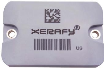
The Xerafy MICRO Paint Shop offers field-proven industrial performance cycling through high temperatures, fluids, and chemicals. The silicone-free design eliminates the risk of contamination in the shop, and the UHF RAIN RFID tag's IP68 rating and survival temperature of 250°C ensure its durability.
