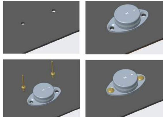
1. Put the tag orientation with symbol "X" in parallel to length of the metal surface.
